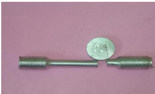
Fig.1 Tensile and hardness specimen
